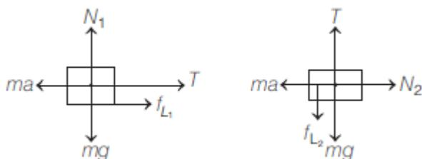
For keeping smaller blocks at rest w.r.t. the bigger block
