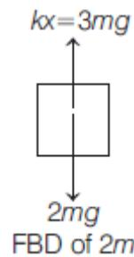
$$\begin{aligned} F &= ma \\ \Rightarrow 3mg - 2mg &= 2ma \\ \Rightarrow a &= \frac{g}{2} \uparrow \end{aligned}$$
