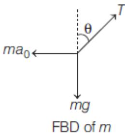
$$\begin{aligned} \sum F_x &= 0 \\ \Rightarrow T \sin \theta &= ma_0 & \dots(i) \\ \sum F_y &= 0 \\ \Rightarrow T \cos \theta &= mg & \dots(ii) \end{aligned}$$
