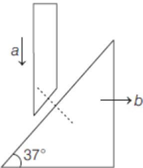
From wedge constraint their acceleration will be same along the common normal at contact.
