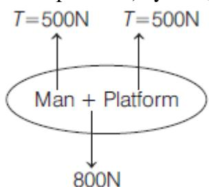
$$\begin{aligned}\sum F_y &= ma_y \\ \Rightarrow 2T - 800 &= 80a \\ \Rightarrow a &= 2.5 \text{ m/s}^2\end{aligned}$$
