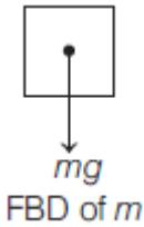
$$\begin{aligned} F &= ma \\ \Rightarrow mg &= ma \\ \Rightarrow a &= g \downarrow \end{aligned}$$
