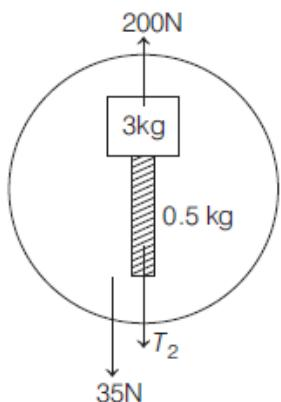
$$\begin{aligned}\sum F_y &= ma_y \\ \Rightarrow 200 - 35 - T_2 &= 3.5(10) \\ \Rightarrow T_2 &= 130\text{ N}\end{aligned}$$
