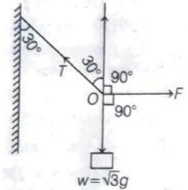
$$\frac{T}{\sin 90^\circ} = \frac{F}{\sin(180^\circ - 30^\circ)} = \frac{w}{\sin(90^\circ + 30^\circ)}$$
