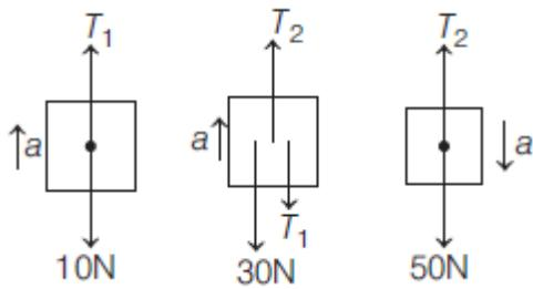
$$50 - T_2 = 5a \quad \dots(i)$$
