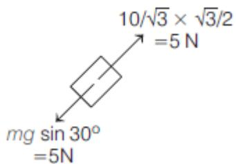
Along the inclined plane, in absence of friction, net force is zero.
