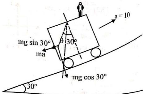
$$\text{From figure, } \tan(30^\circ + \theta) = \frac{mg \sin 30^\circ + ma}{mg \cos 30^\circ}$$
