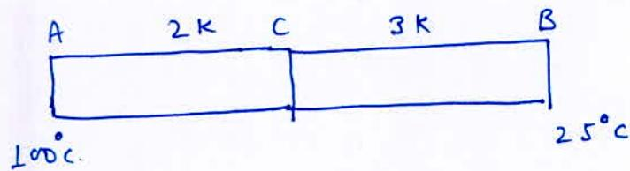
$$q = \frac{\Delta T}{\frac{L}{2KA} + \frac{L}{3KA}} = \frac{6}{5} \frac{\Delta T KA}{L} = \frac{6}{5} \times 75 \frac{KA}{L}$$
