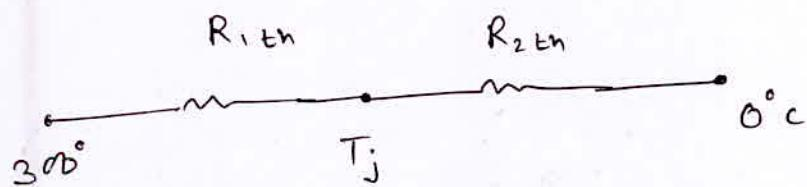
$$q = \frac{300 - 0}{R_1 + R_2} = \frac{300}{\frac{L}{K_A} + \frac{L}{2K_A}}$$
