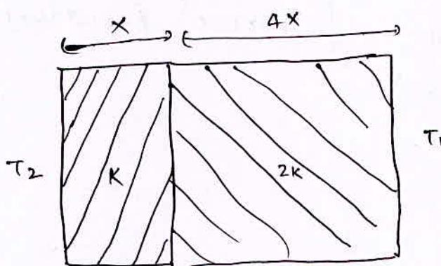
$$\dot{q} = \frac{\frac{T_2 - T_1}{x}}{\frac{K A}{KA} + \frac{\frac{4x}{2KA}}{KA}} = \frac{KA(T_2 - T_1)}{3x}$$
