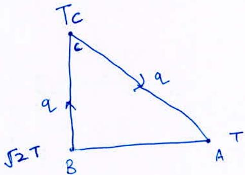
$$\frac{\int_2 T - T_c}{\frac{L}{KA}} = \frac{T_c - T}{\frac{\int_2 L}{KA}}$$
