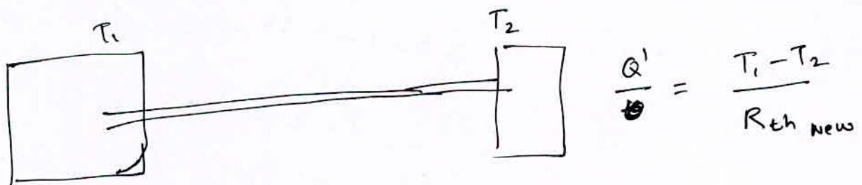
$$\frac{Q'}{t} = \frac{T_1 - T_2}{R_{th, new}}$$
