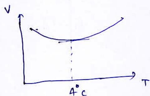
$$\frac{dV}{dT} = 0 \text{ at } 4^{\circ}\text{C} \Rightarrow \gamma = 0$$
