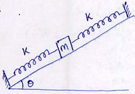
The two springs are in parallel combination because extension in one spring = compression in other
