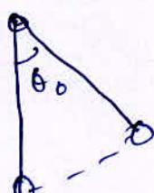
$$T_{\max} = mg + \frac{mv^2}{l}$$
