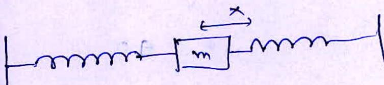
$$F_{net} = 2kn + kn = 3kn$$
