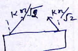
$$\begin{aligned} \text{Frestoring} &= 2 \cos 45^\circ \frac{Kx}{\sqrt{2}} \\ &= kx \end{aligned}$$
