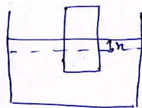
$$T = 2\pi \sqrt{\frac{n}{a}} = 2\pi \sqrt{\frac{\rho_{\text{wood}} a b c}{\rho_{\text{water}} b c g}}$$
