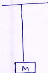
Increased Energy per unit volume =  $\frac{1}{2} \times \text{stress} \times \text{strain}$
