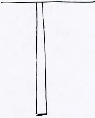
Tension is maximum at top most point. ( $T = mg$ )
