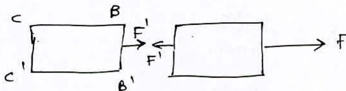
$$F' = \left( \frac{x}{L} \right) M \times a = \frac{x}{L} M \times \frac{F}{M} = \frac{Fx}{L}$$
