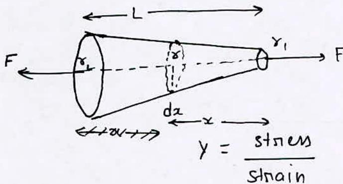
$$\frac{r_2 - r_1}{L - 0} = \frac{r - r_1}{x - 0}$$
