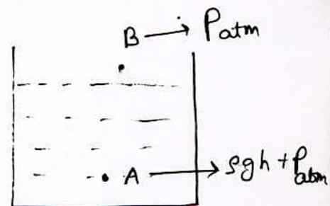
$$\begin{aligned}\Delta V &= - \frac{\Delta P \times V}{k} \\ &= - \frac{\rho g h \times V}{k} \\ &= - \frac{10^3 \times 9.8 \times 200 \times 10^{-6}}{2.2 \times 10^9} \\ &= \frac{19.6 \times 10^{-10}}{2.2} \text{ m}^3 \\ &= 8.8 \times 10^{-10} \times 10^6 \text{ cm}^3 \\ &= 8.8 \times 10^{-4} \text{ cm}^3\end{aligned}$$
