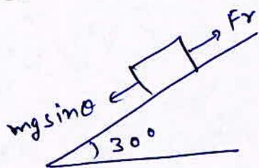
$$\begin{aligned} F_r &= mg \sin \theta \\ &= 2 \times g \times \sin 30^\circ \\ &= g \\ &= 9.8 \text{ N} \end{aligned}$$
