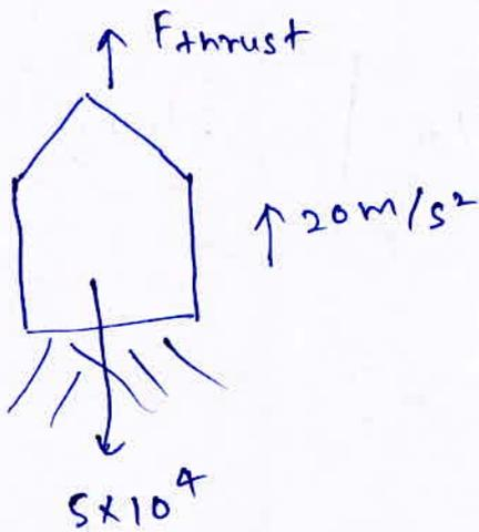
$$F_{\text{thrust}} - 5 \times 10^4 = 5 \times 10^3 \times 20$$
