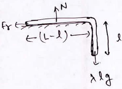
assuming  $\lambda \text{ kg/m}$  is per unit length (mass of chain)
