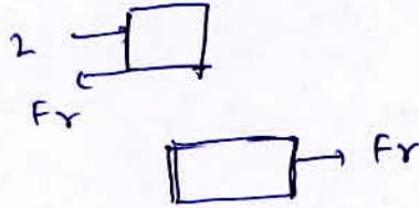
$$\begin{aligned} F_{r \max} &= \mu N \\ &= \frac{1}{4} \times 20 \\ &= 5 \text{ N} \\ a_{\text{trolley max}} &= \frac{5}{20} = 0.25 \end{aligned}$$
