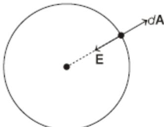
Using Gauss's law,  $\phi = \frac{q_{\text{enclosed}}}{\epsilon_0}$
