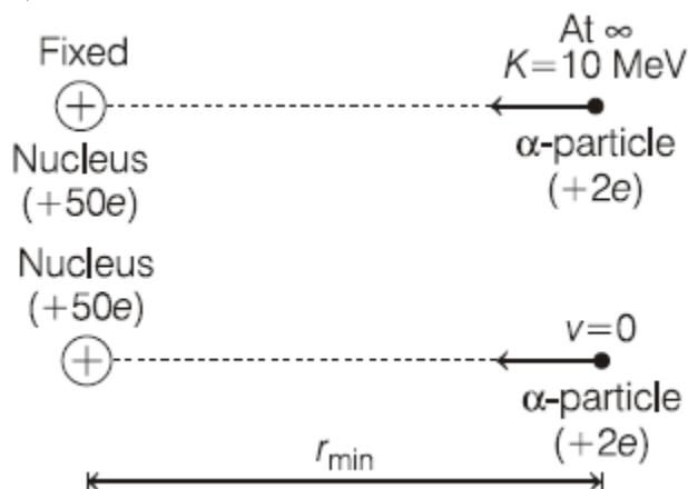
At the minimum distance of approach, speed of  $\alpha$ -particle would be zero.
