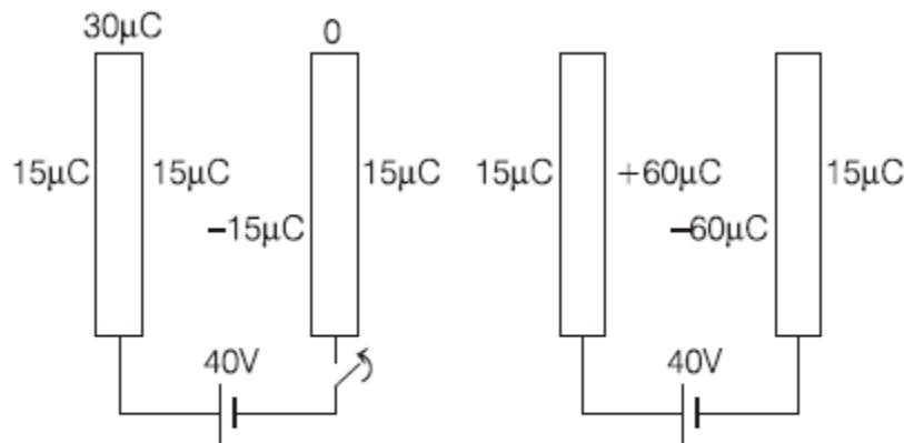
$$\text{Charge flown through battery} = 60 - 15 = 45 \mu\text{C}$$
