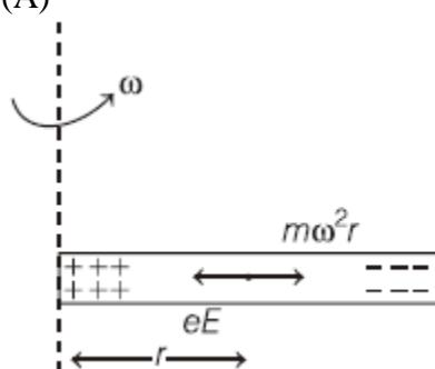
Due to centrifugal force on free electrons, electrons will accumulate at the right end of the rod and there will be deficiency of electrons at the left end. These induced charges will give rise to an electric field.
