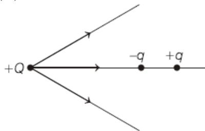
Force on the dipole will be non-zero as electric field produced by a point charge is non-uniform. Torque will be zero, if the dipole is aligned along one of electric field lines as shown in figure. For any other orientation of dipole, torque will be non-zero.
