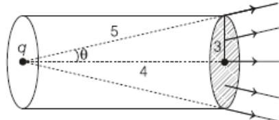
$$\begin{aligned} \text{Flux through the right flat face} &= \frac{q/\epsilon_0}{4\pi} [2\pi(1 - \cos\theta)] \\ &= \frac{q}{2\epsilon_0} \left(1 - \frac{4}{5}\right) = \frac{q}{10\epsilon_0} \end{aligned}$$
