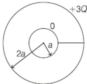
After closing the switch, the entire charge of inner shell will be transferred to the outer shell.
