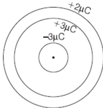
$$\begin{aligned} V &= V_1 + V_2 + V_3 \\ &= \frac{k(-3\mu C)}{(9 \text{ cm})} + \frac{k(+3\mu C)}{(9 \text{ cm})} + \frac{k(+2\mu C)}{(10 \text{ cm})} \\ &= \frac{9 \times 10^9 \times 2 \times 10^{-6}}{10 \times 10^{-2}} \\ &= 180 \text{ kV} \end{aligned}$$
