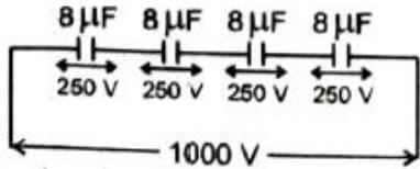
$$\frac{1}{C_{eq}} = \frac{1}{8} + \frac{1}{8} + \frac{1}{8} + \frac{1}{8} \quad \therefore C_{eq} = 2 \mu\text{F}$$
