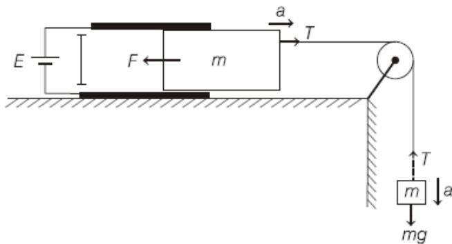
$$mg - T = ma \quad \dots(i)$$
