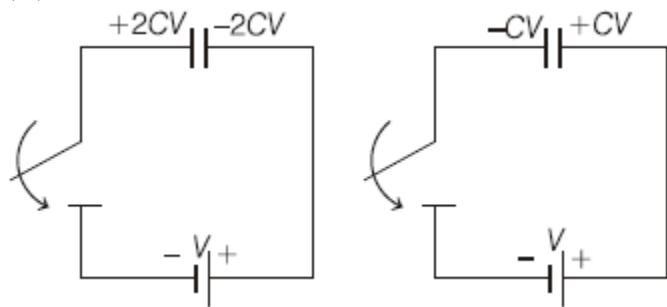
$$\begin{aligned}\text{Charge flown through battery} &= CV - (-2CV) \\ &= 3CV\end{aligned}$$
