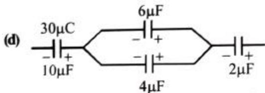
As given in the figure,  $6\mu F$  and  $4\mu F$  are in parallel. Now using charge conservation.
