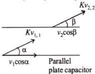
$$\therefore \frac{K_1}{K_2} = \frac{\frac{1}{2}mv_1^2}{\frac{1}{2}mv_2^2} = \frac{v_1^2}{v_2^2} = \frac{\cos^2 \beta}{\cos^2 \alpha}$$
