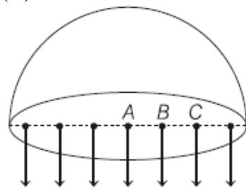
Electric field due to hemisphere at points lying on the diameter is perpendicular to the diameter.
