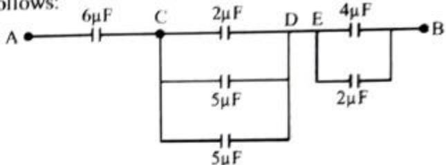
The equivalent capacitance between C & D capacitors of 2 μF, 5 μF and 5 μF are in parallel.
