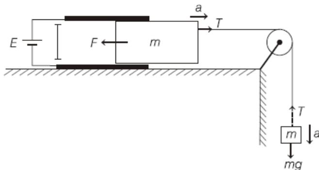
$$mg - T = ma \quad \dots(i)$$
