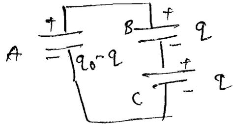
$$U_{\text{system}} = U_A + U_B + U_C = \frac{(Q_0 - Q)^2}{2C_1} + \frac{Q^2}{2C_2} + \frac{Q^2}{2C_3}$$
