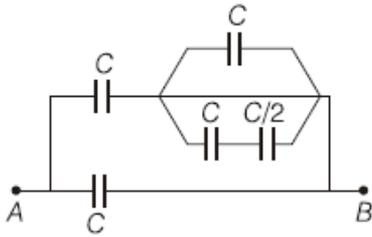
$$C_{eq} = \frac{11C}{7} = \frac{11}{7} (7\mu\text{F}) = 11\mu\text{F}$$
