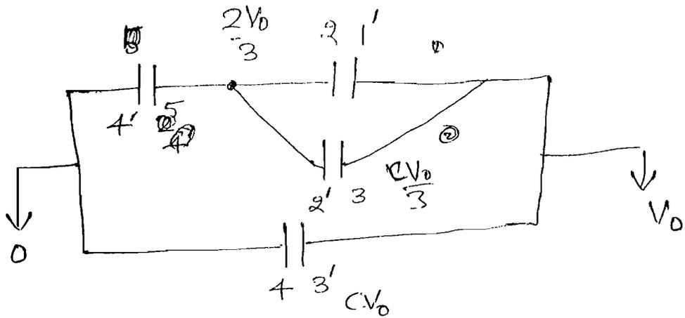
charge on plate 5 =  $\frac{2V_0}{3} \times C = \frac{2 \cdot CV_0}{3}$
