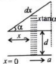
Total capacitance of system can be obtained by integrating with limits  $x = 0$  to  $x = a$
