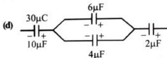
As given in the figure,  $6\mu\text{F}$  and  $4\mu\text{F}$  are in parallel. Now using charge conservation.
