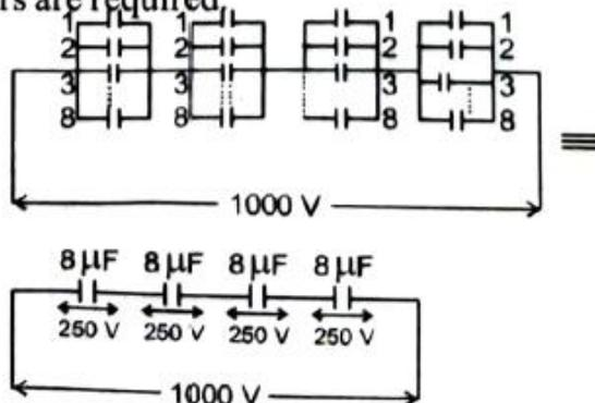
$$\frac{1}{C_{eq}} = \frac{1}{8} + \frac{1}{8} + \frac{1}{8} + \frac{1}{8} \quad \therefore C_{eq} = 2 \mu\text{F}$$
