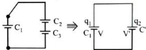
$$\text{As } V = V' \Rightarrow \frac{q_1}{C_1} = \frac{q_2}{C'} \Rightarrow \frac{q_1}{1} = \frac{q_2}{2} \Rightarrow q_1 = \frac{q_2}{2}$$
