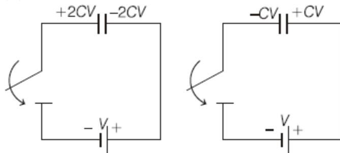
$$\text{Charge flown through battery} = CV - (-2CV) \\ = 3CV$$
