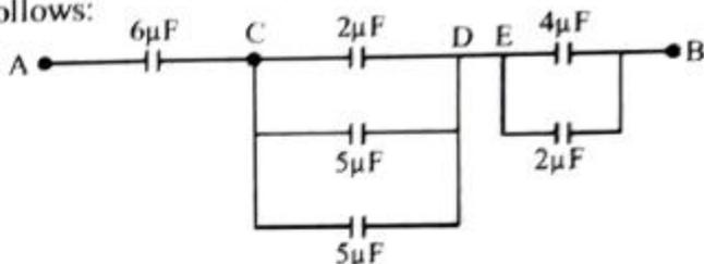
The equivalent capacitance between C & D capacitors of  $2\mu\text{F}$ ,  $5\mu\text{F}$  and  $5\mu\text{F}$  are in parallel.
