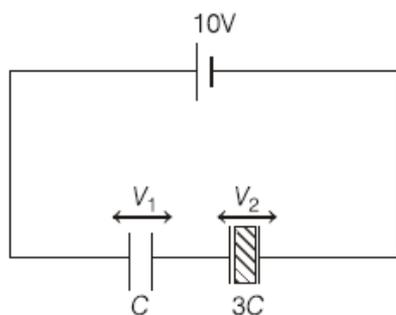
$$V_1 + V_2 = 10 \quad \dots(i)$$
