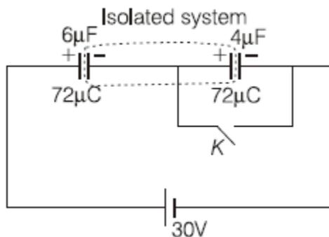
$$C_{\text{eq}} = \left( \frac{1}{6} + \frac{1}{4} \right)^{-1} = 2.4 \mu\text{F}$$
