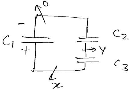
$$\begin{aligned} (x-0)C_1 + (x-y)C_3 &= qV \\ (y-0)C_2 + (y-x)C_3 &= 0 \\ (C_1 + C_3)x - C_3y &= qV \\ (C_2 + C_3)y - C_3x &= 0 \end{aligned}$$
