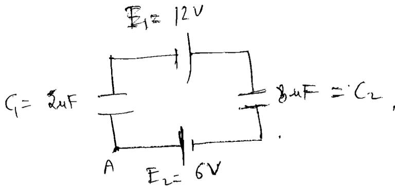
Charge flowing through  $C_1$  and  $C_2$  will be same
