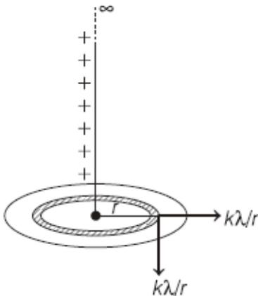
Lets take a ring of radius  $r$  and thickness  $dr$  flux through the ring =  $d\phi$
