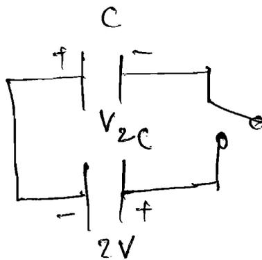
Final common potential  $V_0 = \frac{4CV - CV}{3C}$
