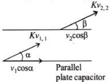
$$\therefore \frac{K_1}{K_2} = \frac{\frac{1}{2} m v_1^2}{\frac{1}{2} m v_2^2} = \frac{v_1^2}{v_2^2} = \frac{\cos^2 \beta}{\cos^2 \alpha}$$
