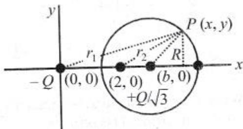
$$V_P = 0 = \frac{k(-Q)}{r_1} + \frac{kQ/\sqrt{3}}{r_2} \Rightarrow \frac{kQ}{r_1} = \frac{kQ/\sqrt{3}}{r_2}$$
