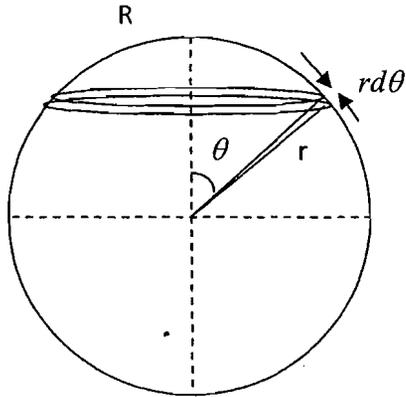
Taking an elemental ring of radius  $r\sin\theta$  and thickness  $rd\theta$ , the area of the sliced portion,
