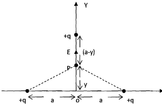
The electric Potential at the point P (0,y) is given by  $V = \frac{1}{4\pi\epsilon_0} \left[ \frac{2q}{\sqrt{a^2 + y^2}} + \frac{q}{(a-y)} \right]$  Therefore the Electric
