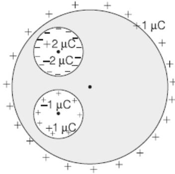
Electric potential at centre of conductor
