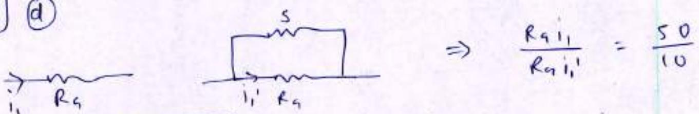
$$\therefore i_1' = \frac{i_1}{5} \quad \therefore R_g \times \frac{i_1}{5} = s \times \frac{q_{11}}{5}$$
