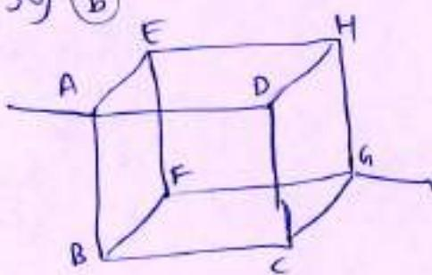
Due to symmetry, points E, O, B will be equipotential and points H, F, C are equipotential.
