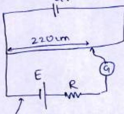
No current here, so the null point does not depend on  $R$
