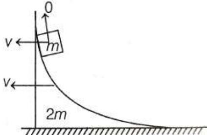
When the smaller block reaches maximum height from ground, its velocity w.r.t. the larger block is zero.
