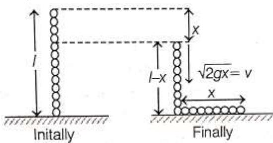
$$F_{\text{Thrust}} = \frac{dm}{dt} v_{\text{rel}} = \frac{d\left(\frac{m}{I}x\right)}{dt} (v - 0)$$
