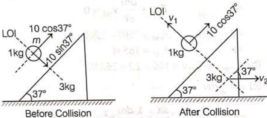
Using conservation of momentum for (wedge + ball) system in horizontal
