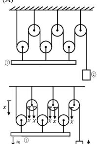
When mass (1) is shifted downwards by x lengths, mass (2) mores upwards by 6x lengths.
