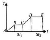
As  $\frac{dT}{dt}$  of CD is smaller, so  $C_{liquid} > C_{solid}$   $Q_1 = H(\Delta t_1)$  and  $Q_2 = H(\Delta t_2)$ AS  $\Delta t_2 > \Delta t_1$ ,  $\therefore Q_2 > Q_1$
