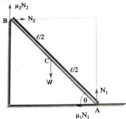
The FBD of the rod is shown in fig. Let  $\theta$  be the angle the rod makes with the horizontal without slipping.
