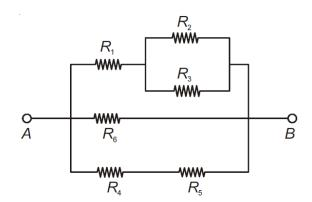
$R_2$  and  $R_3 \Rightarrow \text{Parallel}$
