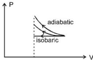
Since area under the curve is max for adiabatic process so work done on the gas will be max for adiabatic process.
